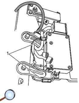
4. Disconnect the cellular antenna and the navigation radio antenna connectors (1).
